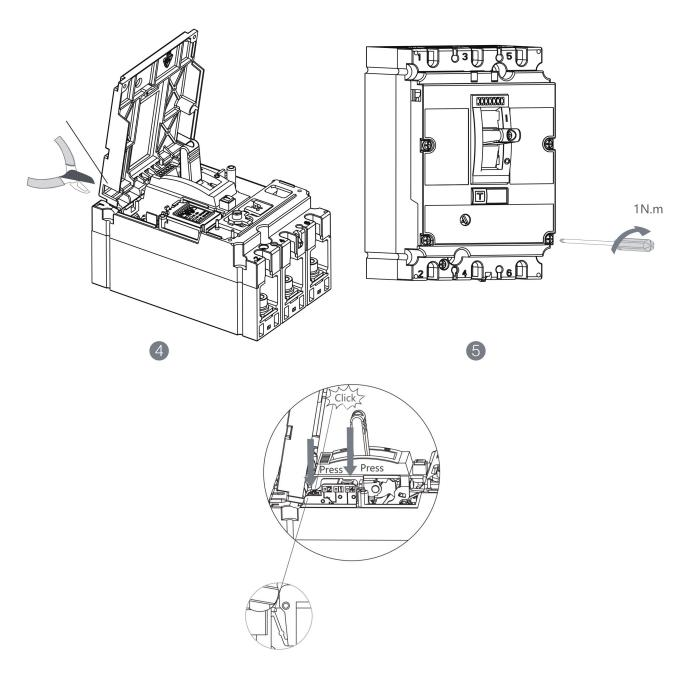
Auxiliary contact-correspondingly installed in the slot marked AX on the circuit breaker
