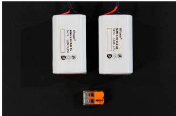
Actual LED-Emergency-Light modules of the type LPU come with two connectors for batteries of 4.8V / 2 Ah.
