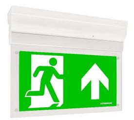
Self-contained Autotest emergency luminaire according to EN 60598-1, EN 60598-2-22, ISO 7010 and EN 1838 for wall-or ceiling mounting. Suitable for maintained and non-maintained operation. Pictogram set (left, right, up, down and white) included. The LED charging indication serves also as test button.
