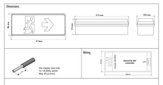
Cable wiring - Connect the mains cable, the LED module to the luminaire using the diagram.
