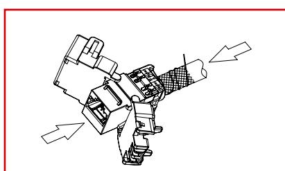
Align the cap with the IDC towers and press it into position.
