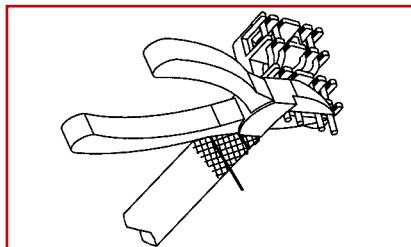
Cut the excess wire off as close to the edge of the cap as possible. Use straight side-cutter.
