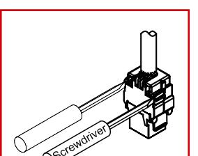
In order to remove the connector clip, insert a small screwdriver into the slot.
