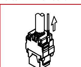
Remove the grounding wire.
