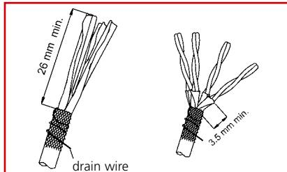
Strip 26 mm of the jacket and fold braid to cover the jacket. Wrap the drain wire around the cable. The foil length of the wires passing are 3.5 mm.
