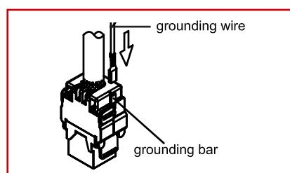
Insert the grounding wire into the grounding bar on the jack.
