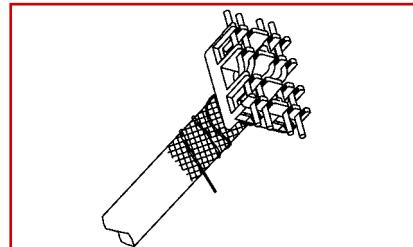
Insert the wires into their correct positions based upon the color code.
