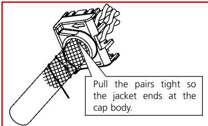
Insert the wires from the stripped cable into the cap through the hole.
