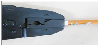
8.Crimp the plug with the crimper
