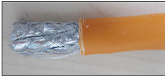
4.Strip the outer Jacket of the raw cable
