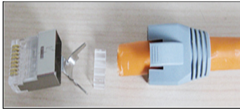
2.Insert the boot to the raw cable
