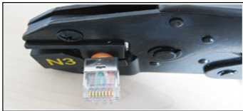
9.Crimp the plug with the crimper
