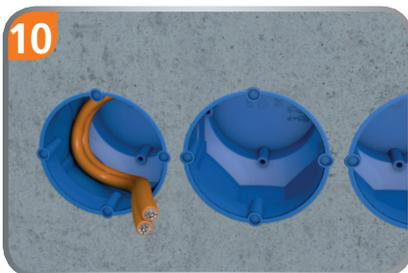
10 **Ideal bending radius:** According to DIN standard for network / Fiber Optic cable
