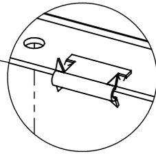
Grounding claws are included in supply of WSA enclosures. Be sure to attach the grounding claw before starting the assembly!
