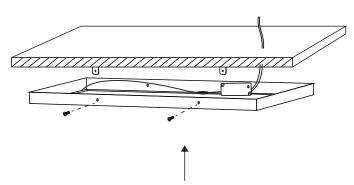
Place the frame on bracket and use screws to fix.
