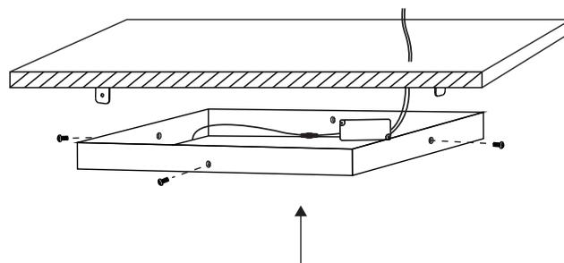
Place the frame on bracket and use screws to fix.
