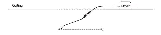
C Install fitting using springs supplied.
