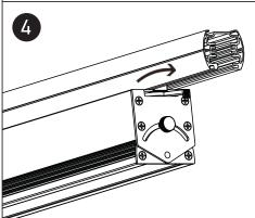
After the track adaptor is inserted, close the security button on the adaptor.
