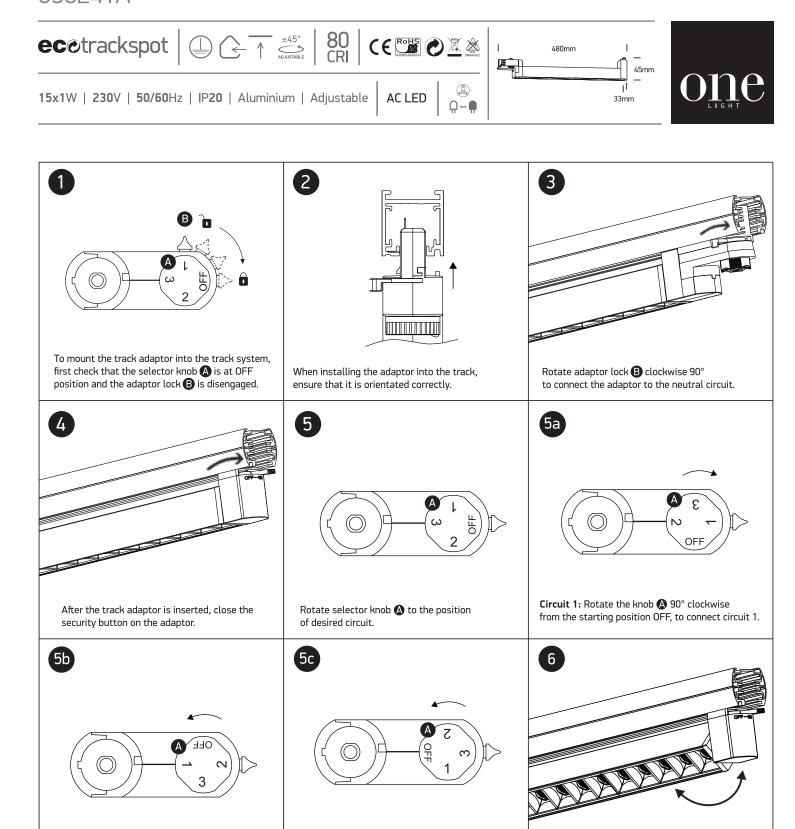
Circuit 3: Rotate the knob (A) 180° clockwise
