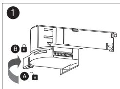
To mount the track adaptor into the track system, first check that the selector knob is at position (A) move to position **B** to lock the adaptor.
