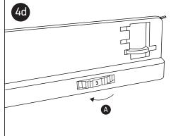
Circuit 3: To connect on circuit 3 rotate the knob (A) to position 3.
