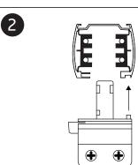
When installing the adaptor into the track, ensure that it is orientated correctly.
