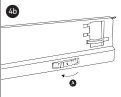
Circuit 1: To connect on circuit 1, from OFF position, rotate the knob  $oldsymbol{A}$  to position 1.
