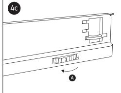
Circuit 2: To connect on circuit 2 rotate the knob (A) to position 2.
