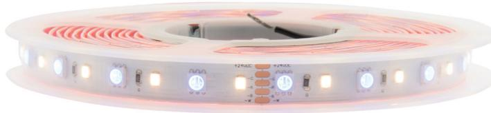
The Flexstrip 86 RGBW has been slightly modified to increase the efficiency of the LED strip, the number of LEDs per meter has been increased from 72 pieces to 84 pieces. The dimensions, the graduation and the lumen output remained the same as well as the article numbers were not changed. As soon as the existing stock levels are used up, only the new version with the white 2835 LEDs instead of the 5050 LEDs will be delivered.
