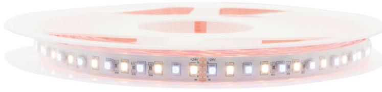
5m reel LED Flexstrip with 50cm long connecting cable at the beginning and end of the strip, with 0.75mm<sup>2</sup> cable cross section. Strip encased in a highly transparent heat shrink pipe with TESA double-sided adhesive tape on the back. Each package includes a 10cm long piece of heat shrink pipe with hot melt adhesive, to seal the end and the beginning of the strip after the assembling.
