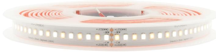
For operation, a supply voltage of min. 23V required. Each segment may be operated with a maximum of 2x35mA, through parallel connection the currents add up. If the luminous flux listed in the table is not 100% required, the Flexstrip CC can also be supplied with lower currents, which also reduces the connected load. **When using appropriate power supplies, a flicker-free amplitude dimming is possible.**
