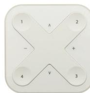
The preset buttons of basicDIM Wireless Interface can be configured via the control app:
