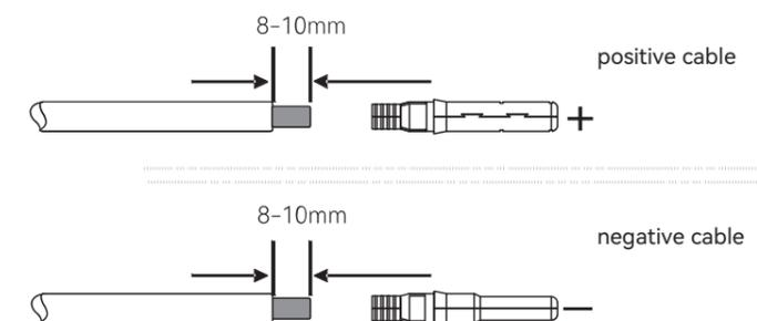
3. Assembly the positive and negative cables with corresponding crimping pliers.
