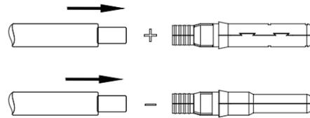
4. Insert the positive and negative cable into positive and negative connector. Gently pull the cables backward to ensure firm connection.
