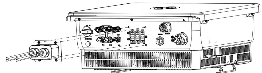
Open the waterproof cover, pass the prepared communication cable through each component, insert corresponding communication port, then tighten the screws.
