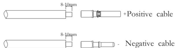
2. Feed the positive and negative cables into corresponding lock screws and crimp them tightly with a wire crimper. Make sure that the withdrawal force of the pressed cable is larger than 400N.
