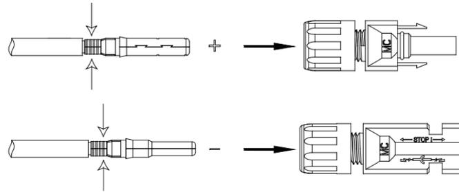
5. Fasten the lock screws on positive and negative connectors.
