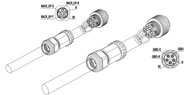
1. Open the waterproof cover, feed the AC cable through the AC waterproof hole.
