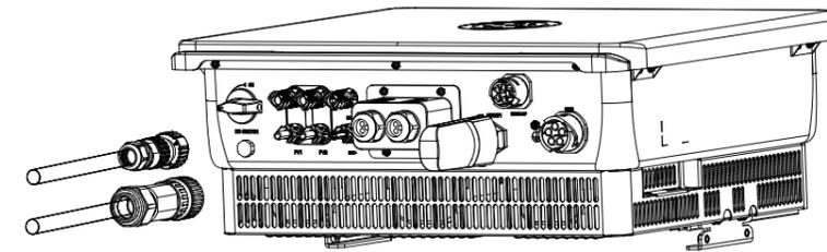
3. Secure all parts of the grid and backup connector tightly.
