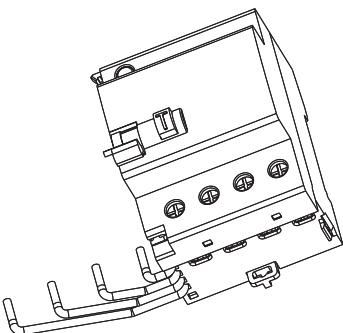
Assembled with NB1, NB1L can offer leakage current protection for human body, and insulation fault protection for electrical equipment.
