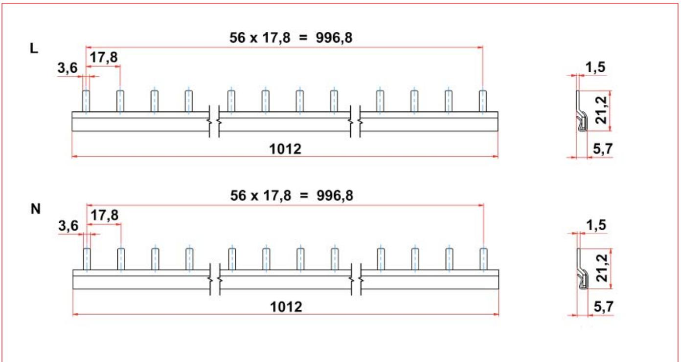
Busbar sets 1-pole+N for miniature circuit breakers 1+N, 1 MW
