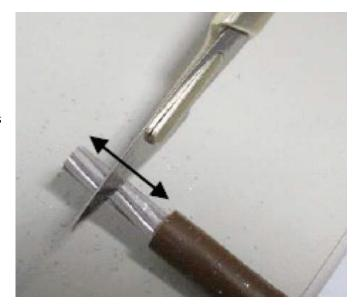
2. After removing the layer of oxide, coat the end of the conductor immediately with a neutral grease, e.g. acidand alkali-free Vaseline, and connect it to the terminal immediately.
